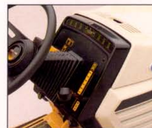
The Super Garden Tractor dash is user friendly. Backlit indicators provide valuable information while operating.
