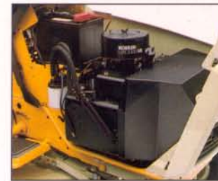
Models 1862 and 1860 are powered by the rugged, 18 HP twin-cylinder Kohler Magnum engine.
