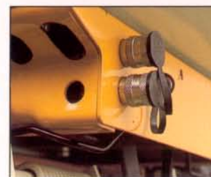
Dual hydraulic front outlets allow for power-assisted attachments. (Hydraulic Outlet Kit: Part No. 759-3493)
