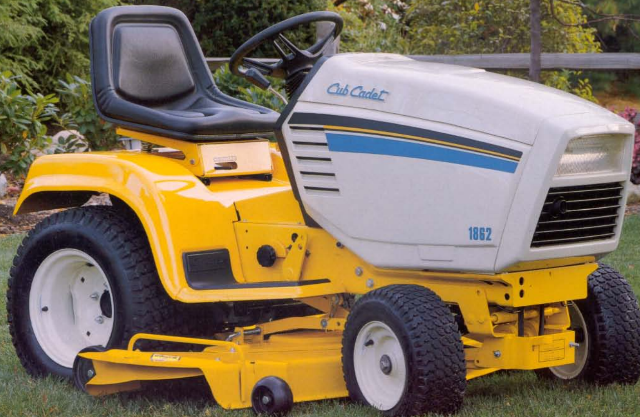
Model 1862 Garden Tractor 18HP / Hydrostatic Transmission / Optional 50" Cutting Deck
