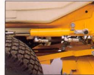
Power steering is standard on Super Garden Tractors.
